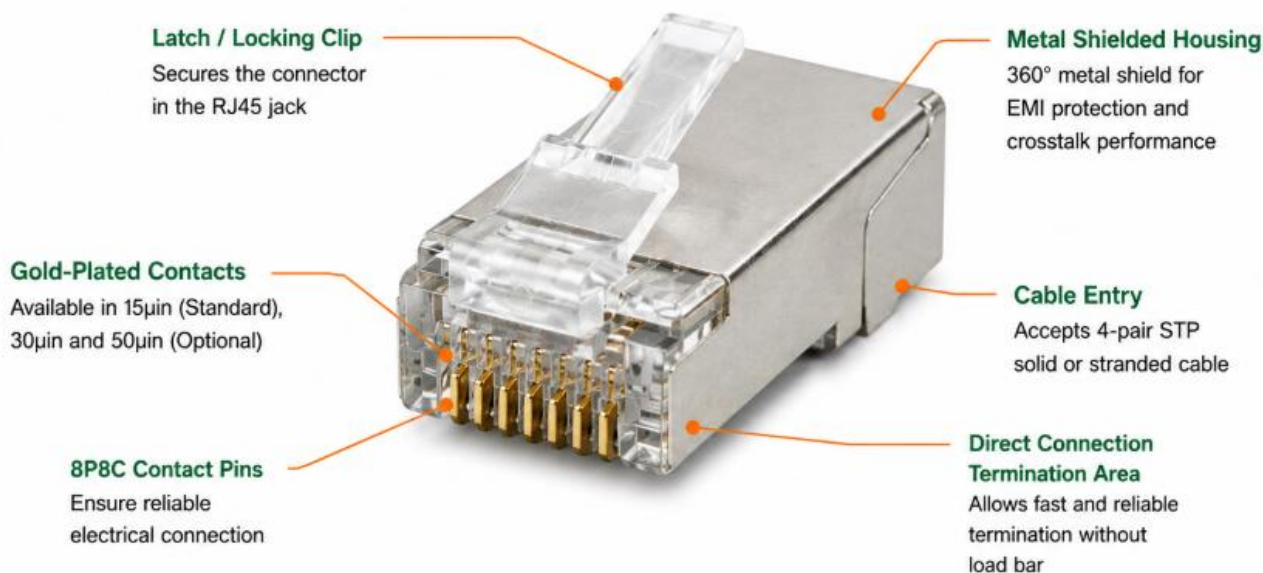
CAT6/6A STP RJ45 Connector - Annotated 3D View
