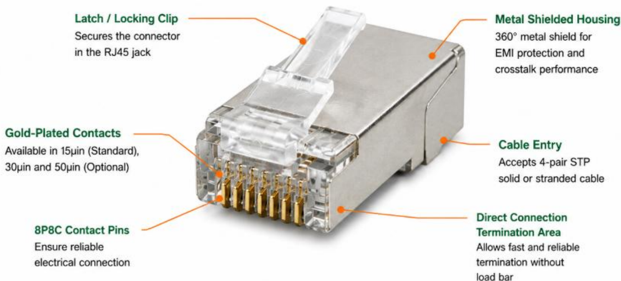
CAT6/6A FTP RJ45 Connector - Annotated 3D View
